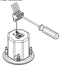
5.3 After the step1 and 2, put the unit into the ceiling round hole after inserting the input connector into the connecting socket.
